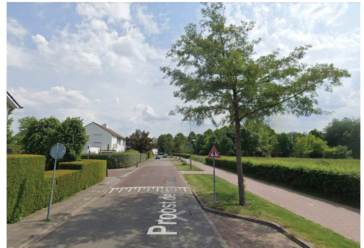
Figure 11: Elevated platform for improved crossing | Meerssen, NL (Source: Google maps street view)
